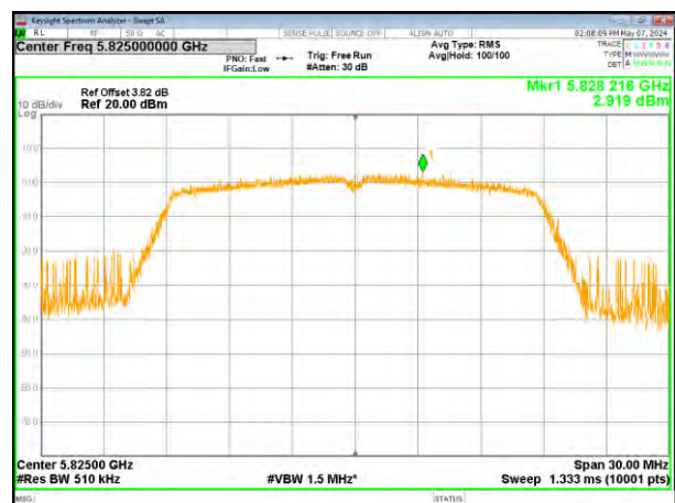
(802.11n20) PSD plot on channel 165
