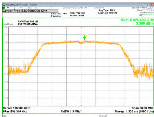
(802.11a) PSD plot on channel 165
