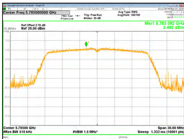
(802.11ac20) PSD plot on channel 157
