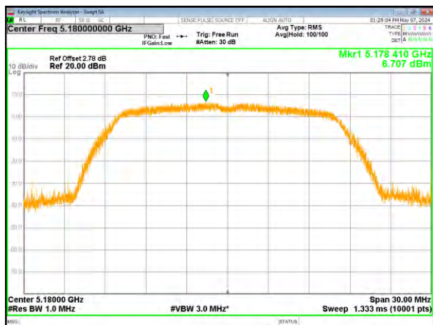
(802.11a) PSD plot on channel 40
