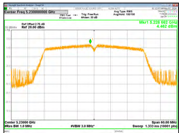
(802.11n40) PSD plot on channel 46
