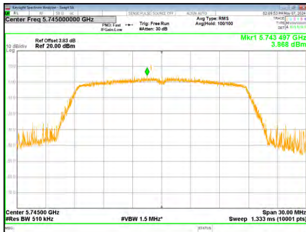
(802.11ac20) PSD plot on channel 157
