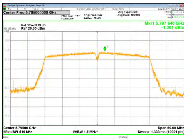
(802.11ac40) PSD plot on channel 159
