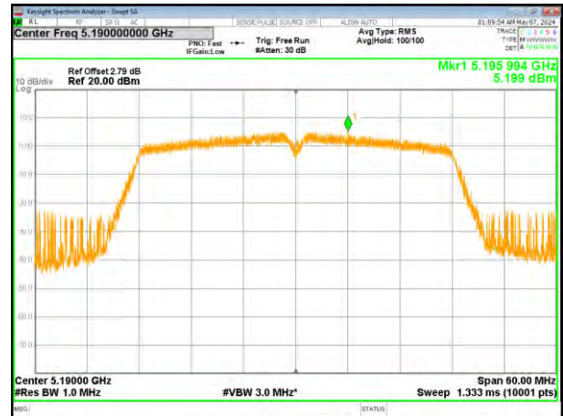
(802.11n40) PSD plot on channel 46
