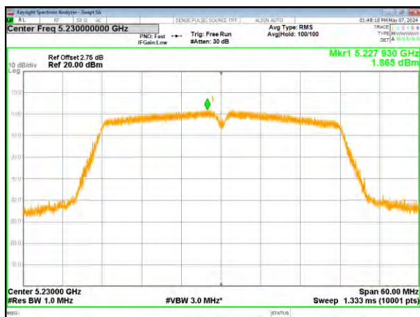
(802.11ac40) PSD plot on channel 46
