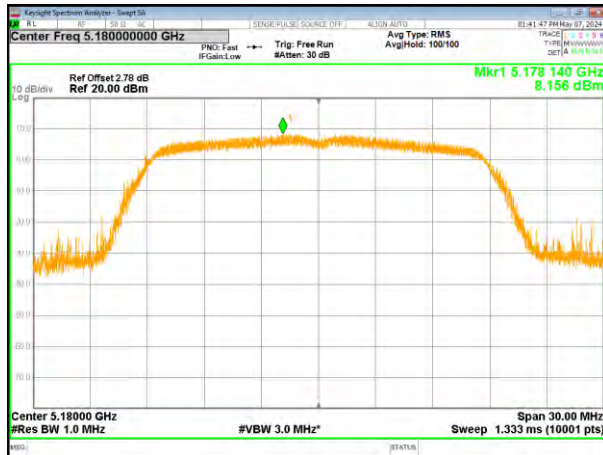
(802.11ac20) PSD plot on channel 40
