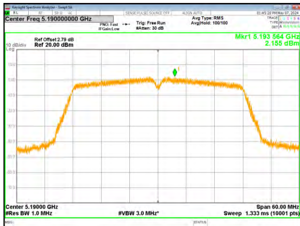
(802.11ac40) PSD plot on channel 46
