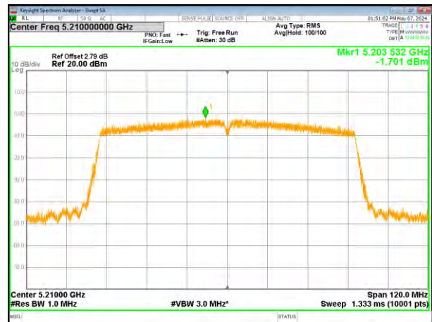
(802.11ac80) PSD plot on channel 42
