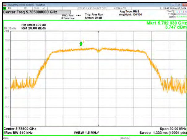
(802.11a) PSD plot on channel 157
