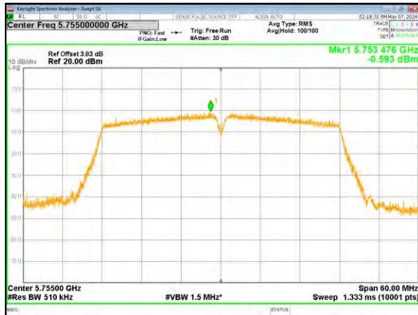
(802.11ac40) PSD plot on channel 151
