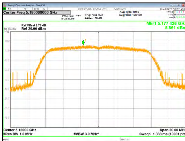
(802.11n20) PSD plot on channel 40
