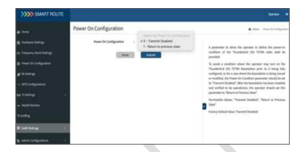
Initially, the power on condition is set to "transmit disabled" on your Thunder 255. This ensures that the TETRA base station does not go online before the carriers are configured. Once the carriers are configured, set to "Return to the previous state" to assure operation resumes after a power outage.
