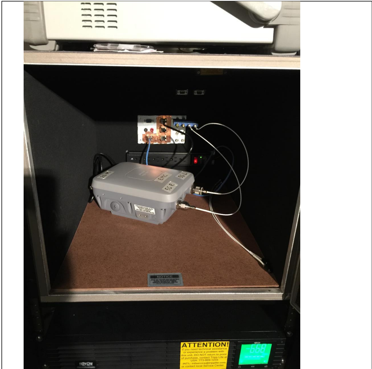
Title: AIR-CAP1532E-B-K9 Conducted Test Setup
