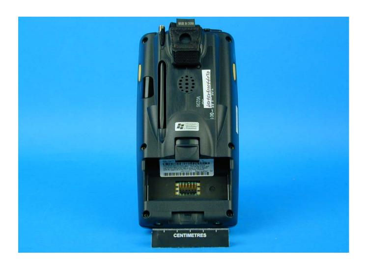
700C-SMC45 Rear (battery removed)
