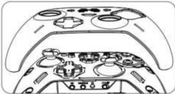
① Open the shell along the bottom seam position.
