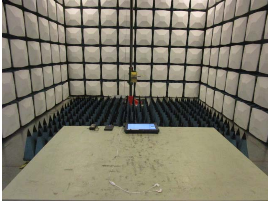
Radiated Emission - Rear View (Above 1GHz)
