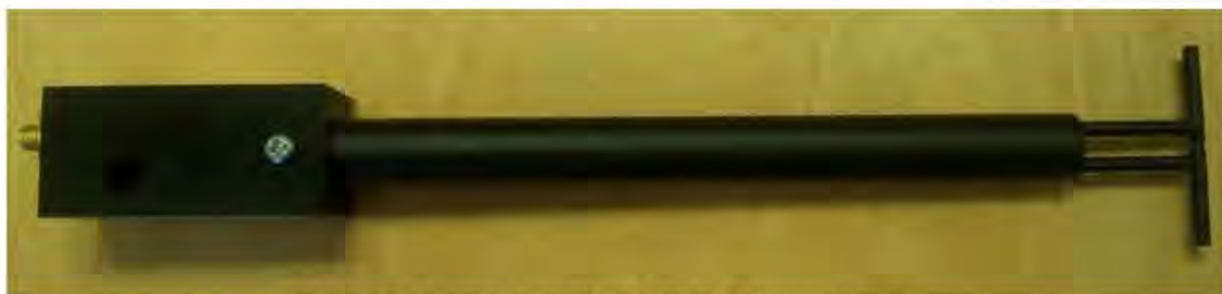
Figure 1 – MVG COMOSAR Validation Dipole
