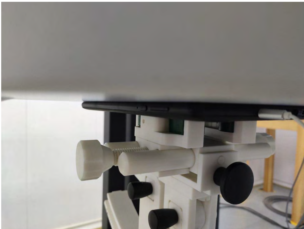
0mm body-worn Front Side Setup Photo (hotspot)
