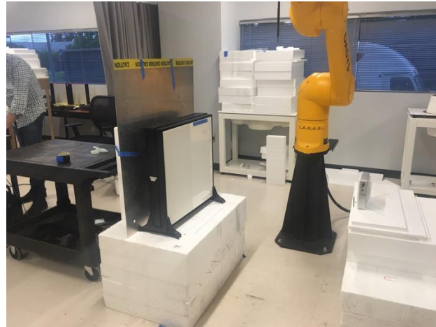
Figure 37: Test setup - metal plate behind WPT Source
