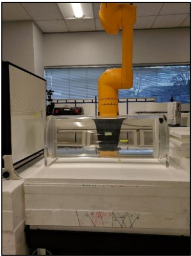
Figure 48 - Test setup - single longitudinal phantom, horizontal plane
