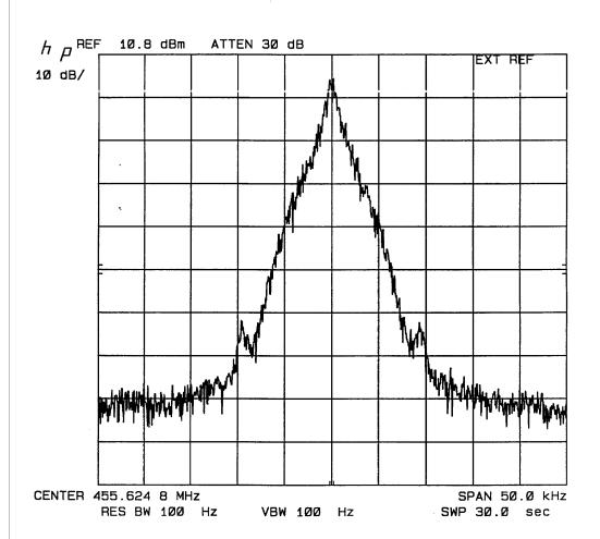
Referenced to the Unmodulated Carrier Modulated with Pseudorandom Data 9600 BPS
