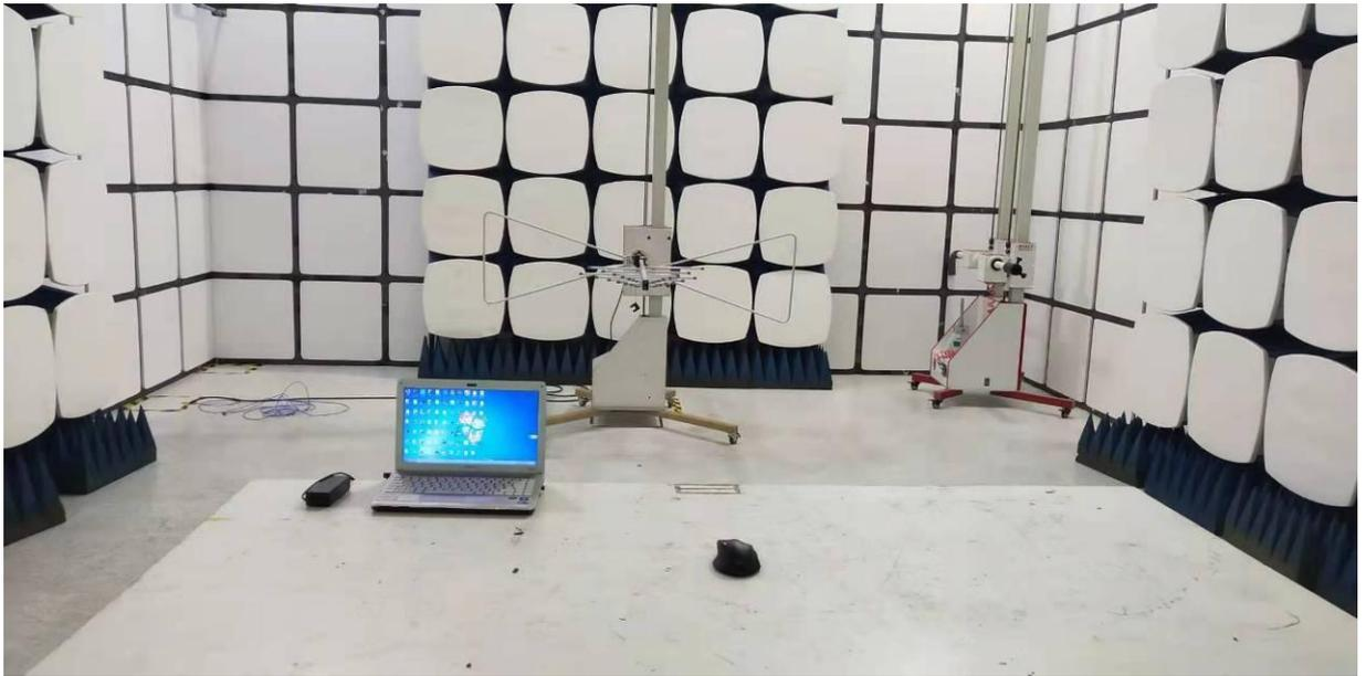
Test frequency from 1GHz-18GHz
