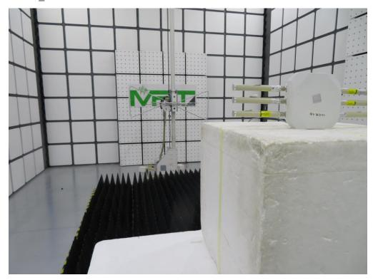
Description: Radiated Spurious Emissions Test Setup for above 1GHz\_OAW-AP1362
