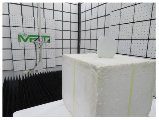
Description: Radiated Spurious Emissions Test Setup for above 1GHz\_OAW-AP1361
