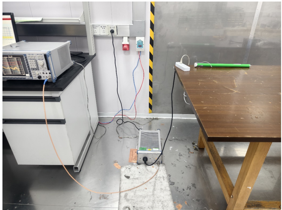
Conducted Emission Test Setup
