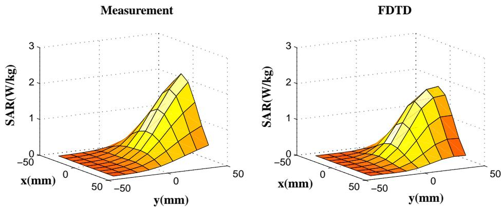
Figure 11. Local SAR in the plane  $d_1=50$  mm for the right translated antenna position at  $h=0$  mm. The maximum and the mean differences between the measurement and the FDTD computation are 0.4 W/kg and 0.1 W/kg.
