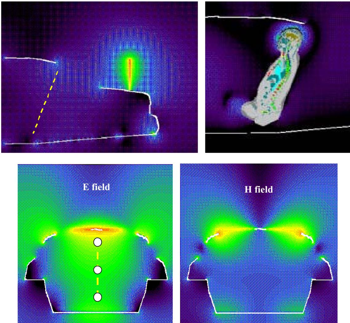
The highest exposure occurs in the middle of the backseat, which is also the case in the measurements. Therefore, the field values were determined on the yellow line centered at the middle of the backseat, approximately at the three locations that are shown by white dots. In actuality, the line is inclined so as to follow the inclination of the passenger's back, as shown previously.
