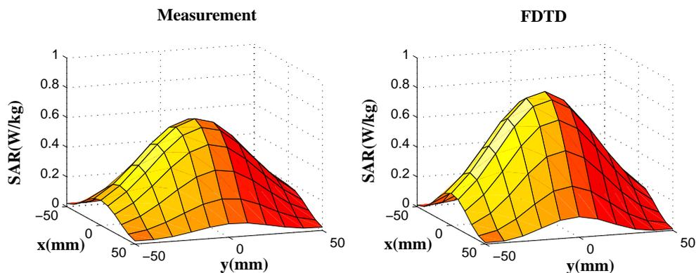
Figure 10. Local SAR in the plane  $d_1=50$  mm for the center antenna position at  $h=5$  mm. The maximum and the mean differences between the measurement and the FDTD results are 0.2 W/kg and 0.06 W/kg.
