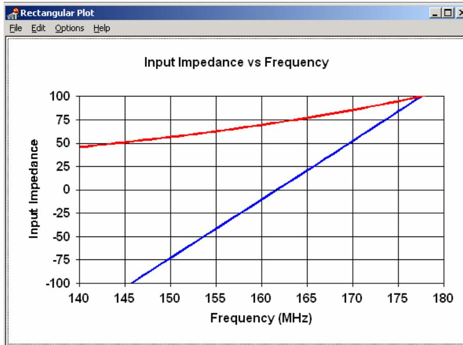
This validation ensures that the input impedance calculation is carried out correctly in XFDTD™, thereby enabling accurate estimates of the radiated power. It further ensures that the wire model employed in XFDTD™, which we used to model the antennas, produces physically meaningful current and fields distributions. Both these aspects ensure that the field quantities are correctly computed both in terms of absolute amplitude and relative distribution.
