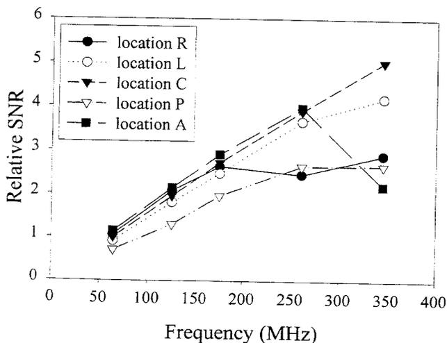
FIG. 7. Line plot of relative SNR at several locations as a function of  $B_1$  frequency when the flip angle is  $90^\circ$  at location C. Locations are 2 cm anterior (location A), posterior (location P), left (reader's right: location L), and right (location R) compared to the point at the center (location C), which is shown in Fig. 4 and was used as the reference for results presented in Figs. 3-6 and Tables 1-2.
