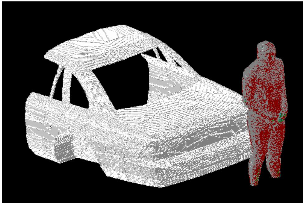
The car model does not include wheels in order to reduce its complexity. The pavement has not been included in the model. The passenger model was validated for similar antenna and frequency conditions by comparing the MPE measurements at one VHF frequency (164 MHz) for a 42 cm monopole antenna used for a VHF mobile radio analyzed previously (FCC ID#ABZ99FT3046). The results are presented below, according to following definitions for the equivalent power densities (based on E or H-field):
