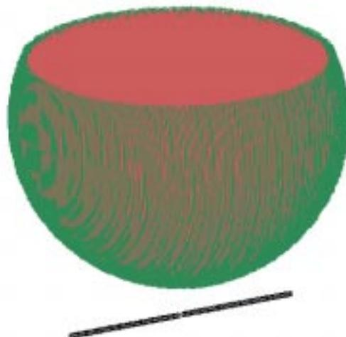
Figure 4. The FDTD models of the spherical bowl and the  $\lambda/2$  dipole. The dipole is placed as centered 25 mm below the outer south pole of the bowl.
