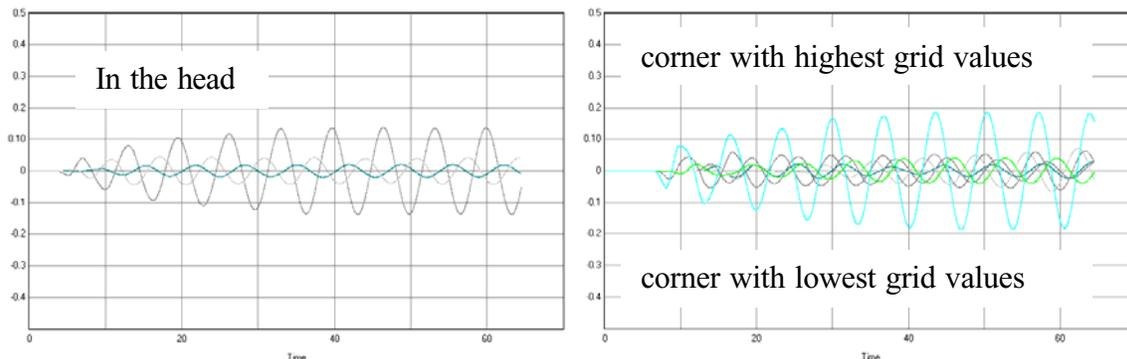
b) 6000 or 6700 (for bystander) time steps were used, with a time step approximately equal to 10 *ps* (meeting the Courant criterion), which corresponds to approximately 9 wave cycles at 149 MHz. Bystander case involves more steps because the simulation domain is larger.
