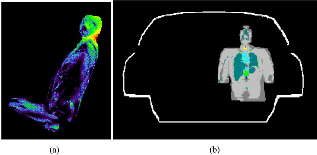
Figure 5: SAR distribution in the passenger model through the plane where the peak SAR occurs (a) placed laterally in the back seat (b), with a trunk-mount antenna operating at 149 MHz.
