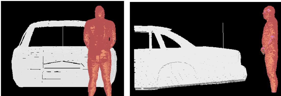
**Figure 1: Bystander model exposed to a trunk-mount quarter wave antenna operating at 149 MHz (a) back view and (b) side view. The antenna is mounted in the center of the trunk. The bystander model is positioned along a 45 deg. line with respect to the longitudinal centerline of the car.**
