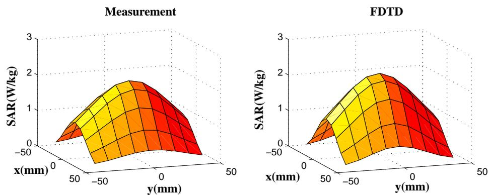
Figure 9. Local SAR in the plane  $d_1=30$  mm for the center antenna position at  $h=5$  mm. The maximum and the mean differences between the measurement and the FDTD computation are 0.3 W/kg and 0.1 W/kg.
