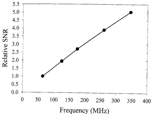
FIG. 6. Line plot of relative SNR as a function of  $B_1$  frequency. Values are normalized to that at 64 MHz. A straight line passed through the two lowest-frequency points and extended towards the origin will very nearly pass through the origin. This suggests good agreement with theory and experiment at low frequencies (1-3).
