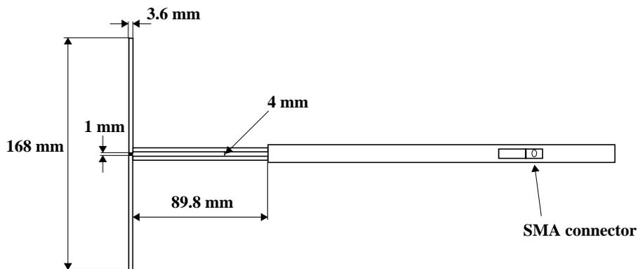
Figure 2. The 835 MHz  $\lambda/2$  dipole used in the measurements. The antenna was manufactured by Schmid & Partner Engineering AG with the model number D835V2 (S/N:401).
