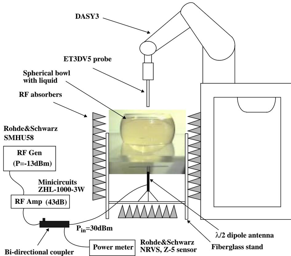
Figure 3. The laboratory setup for the IEEE SCC 34 spherical bowl and dipole experiment.
