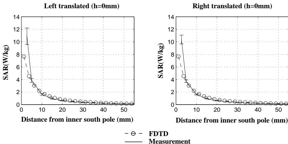
**Figure 8.** The measured and the FDTD computed SAR on the axis of symmetry for the spherical bowl. The half-wave dipole antenna was placed 0 mm below the outer south pole and translated to the left and right side.
