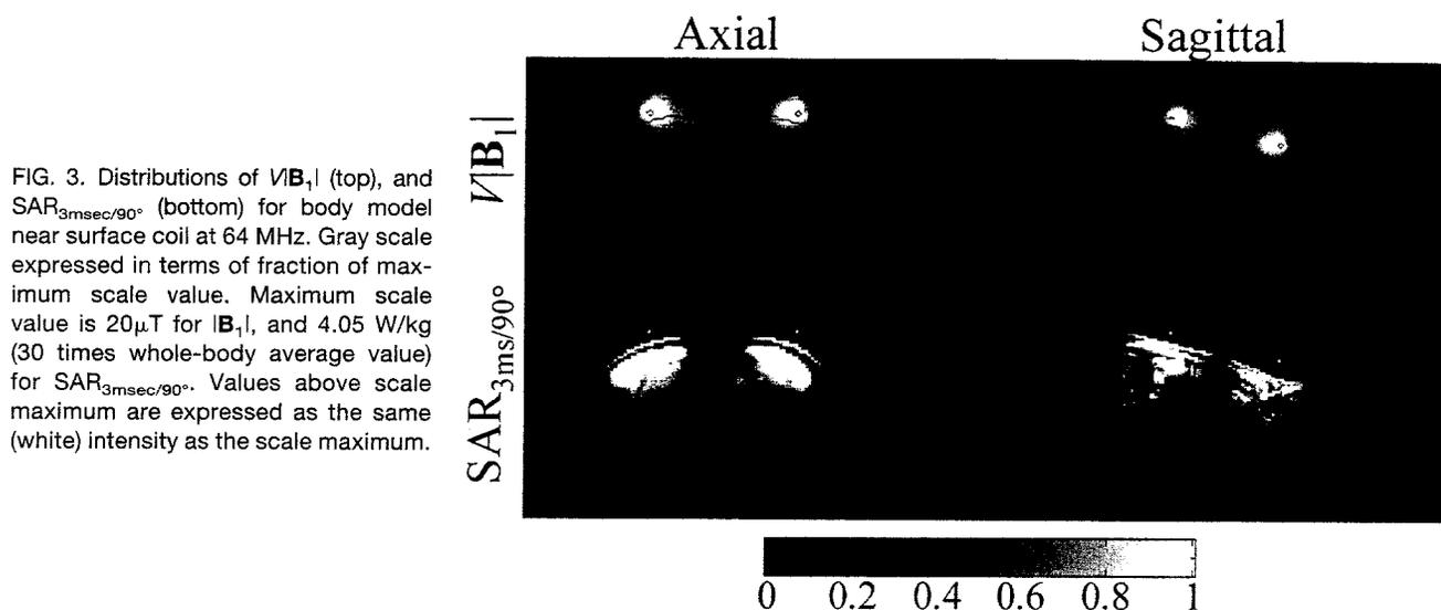
FIG. 3. Distributions of  $V|B_1|$  (top), and  $SAR_{3msec/90^\circ}$  (bottom) for body model near surface coil at 64 MHz. Gray scale expressed in terms of fraction of maximum scale value. Maximum scale value is  $20\mu T$  for  $|B_1|$ , and  $4.05 W/kg$  (30 times whole-body average value) for  $SAR_{3msec/90^\circ}$ . Values above scale maximum are expressed as the same (white) intensity as the scale maximum.
