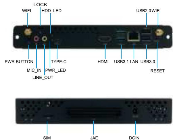
**Note:** This illustration is for reference only, which may be different from the material object. The definition of all the jumpers and sockets which are marked in the above picture, please refer to the following "Interface Instructions" part.
