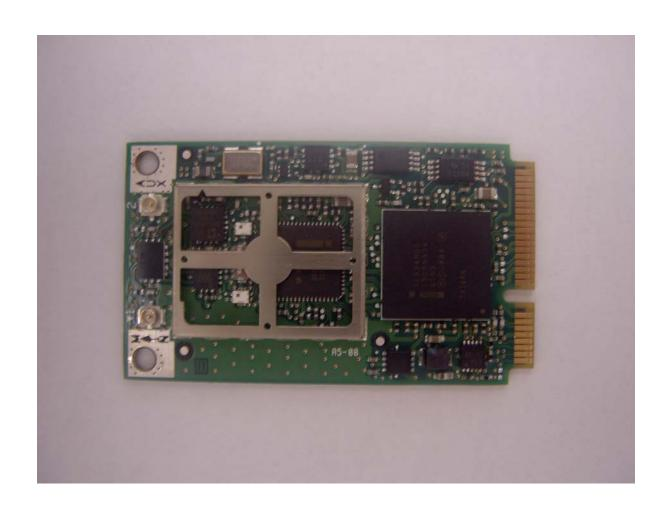
Top View "Shielding removed"
