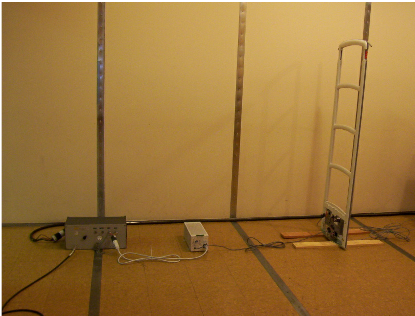
Photo 1 – LIBERTY DX – CONDUCTED EMISSIONS TEST SETUP
