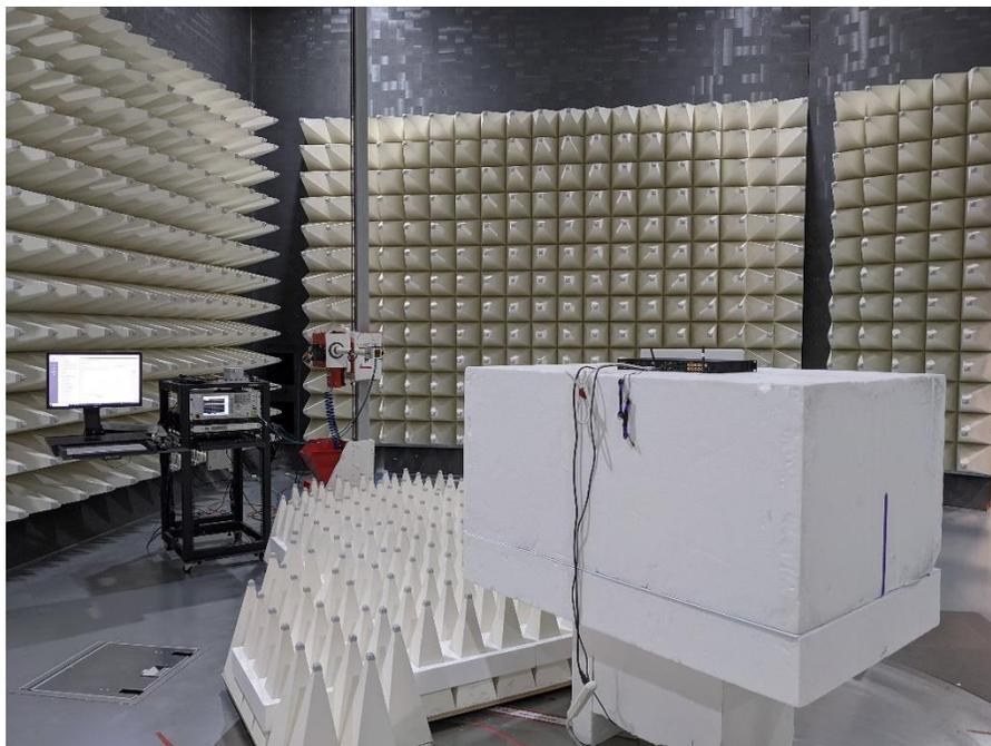
**Photograph 3: Radiated Emissions 17 - 26 GHz**
