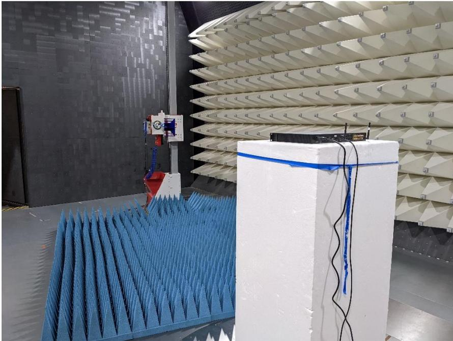
**Photograph 2: Radiated Emissions 1 - 17 GHz**
