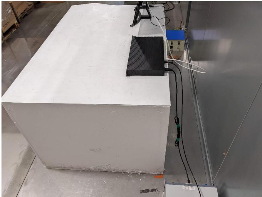
**Photograph 6: Test Set Up AC Mains Conducted Emissions**
