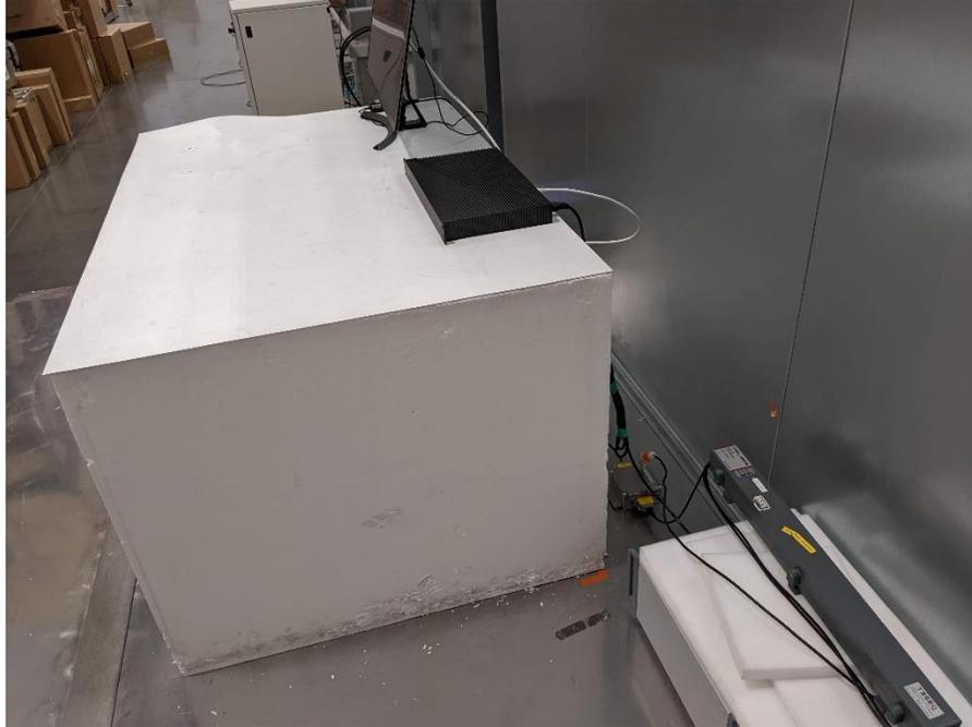
**Photograph 5: Test Set Up AC Mains Conducted Emissions**
