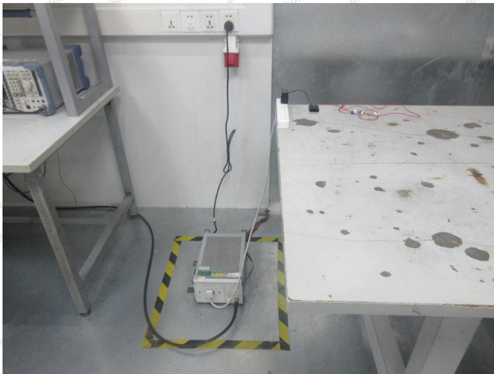
Photo of Conducted Emission Measurement
