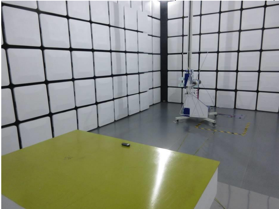
RADIATED RF MEASUREMENT SETUP (30MHz ~ 1 GHz - Z axis)
