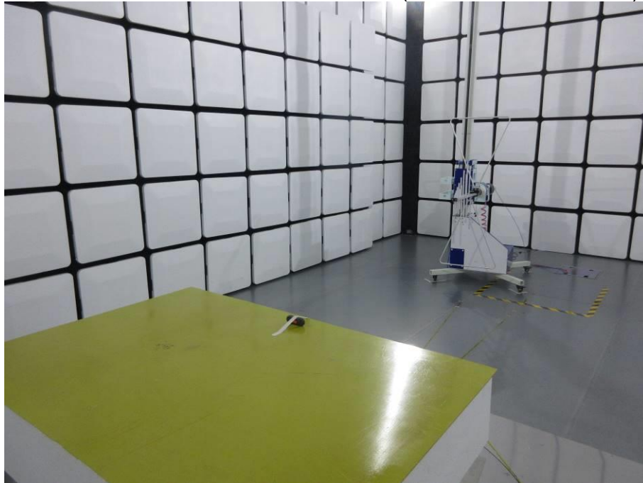
RADIATED RF MEASUREMENT SETUP (30MHz ~ 1 GHz - X axis)
