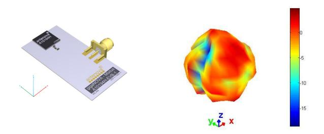
**3D pattern at 5500 MHz**Drag to rotate pattern and PCB by using Adobe Reader
