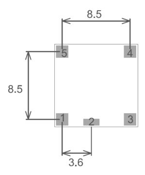
PADS 1,3,4,5 = 1.5 X 1.5 (MM) PAD 2 = 2.0 X 0.8 (MM) ALL DIMENSIONS IN MM
