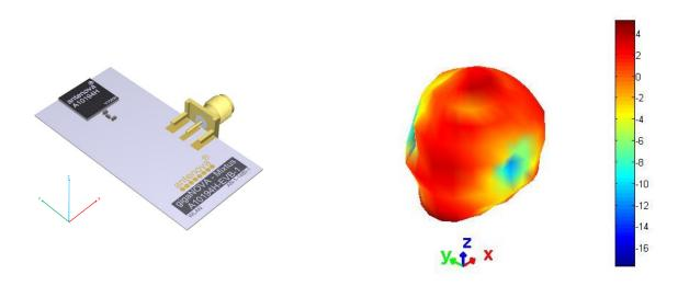
**3D pattern at 2450 MHz**Drag to rotate pattern and PCB by using Adobe Reader
