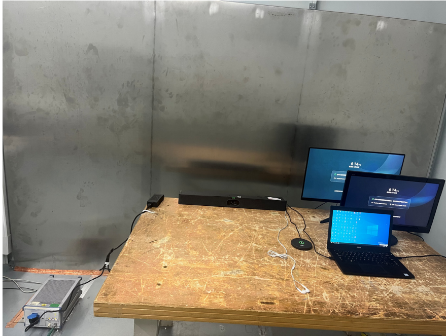
Conducted Emissions - Side View
