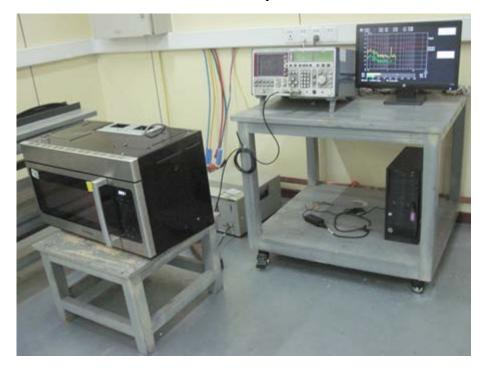
Radiated Emission Test Set-up (30 -1,000MHz):
