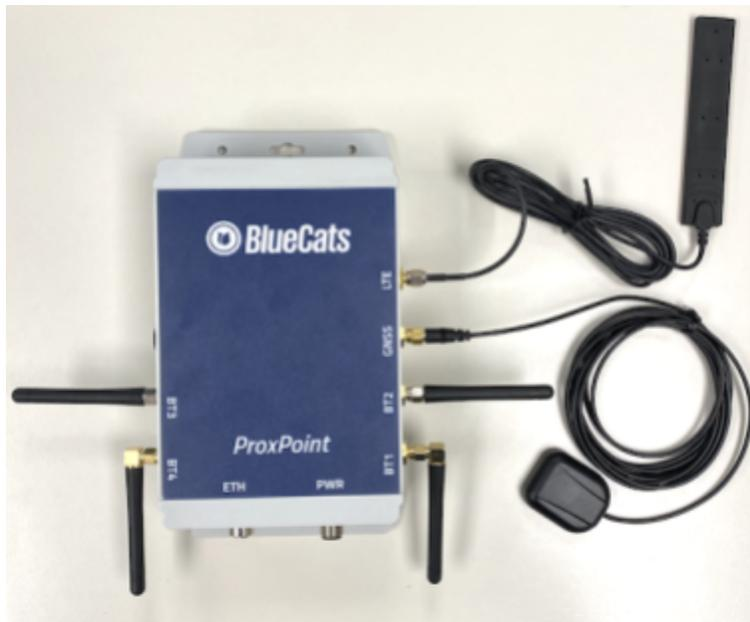
**Figure 3.** ProxPoint with all antennas attached.
