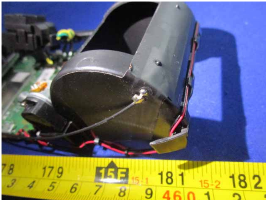
EUT- UMTS Antenna View
