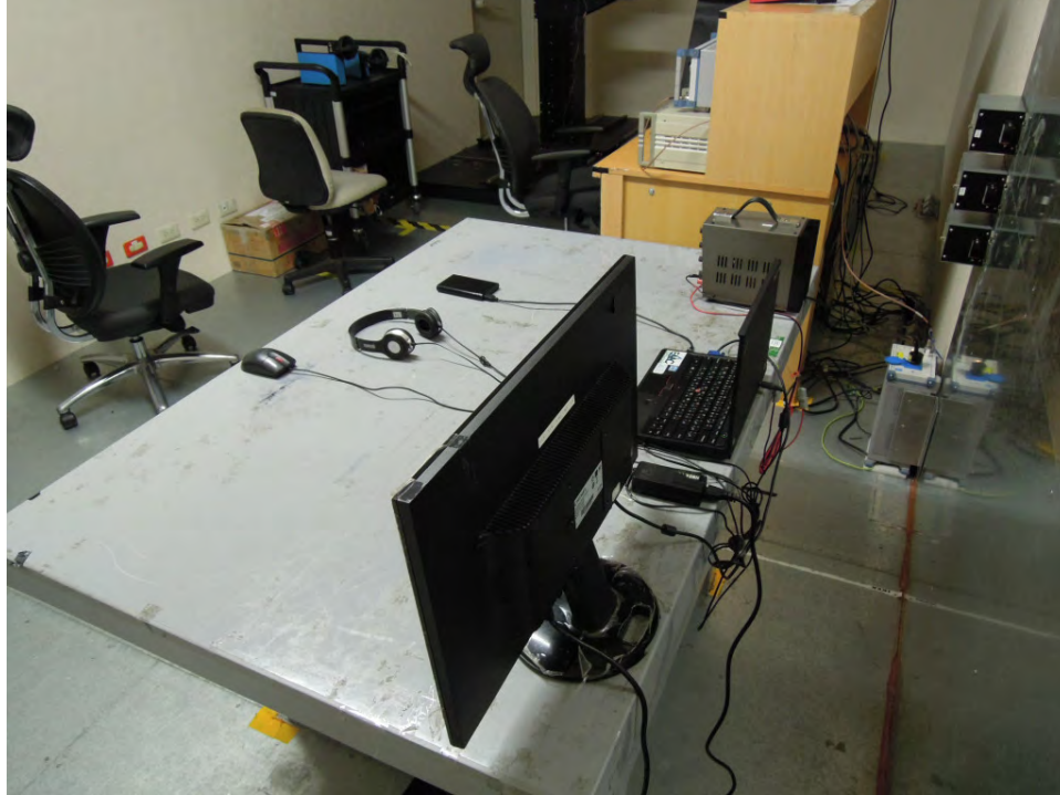
Photograph 7: Set-up for Mains Conducted testing (Back View)
