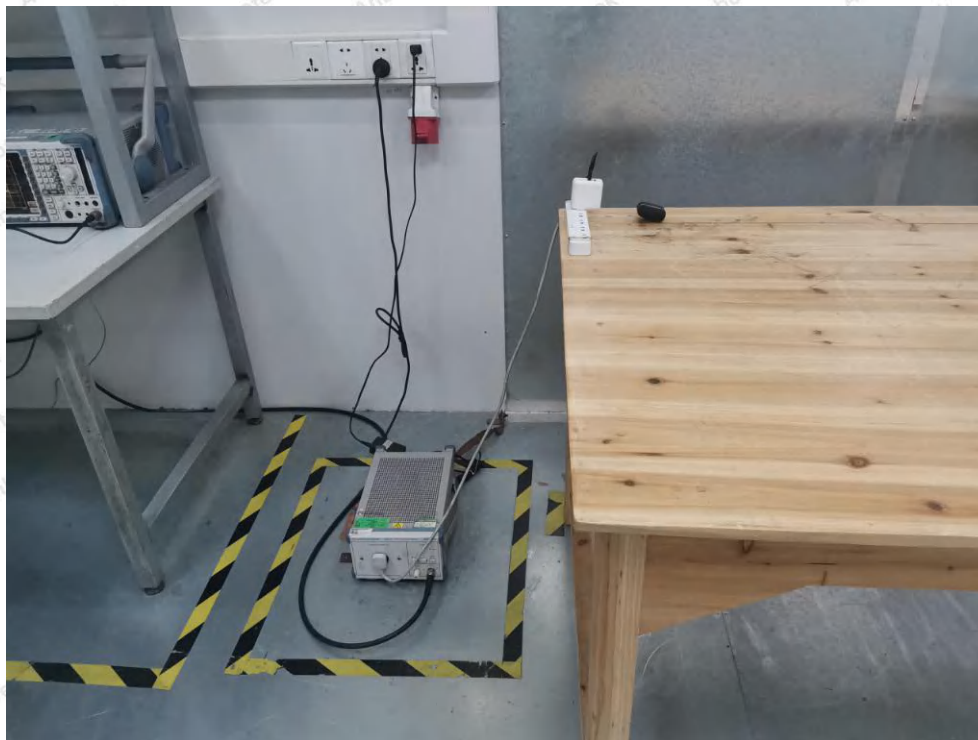
Photo of Conducted Emission Measurement
