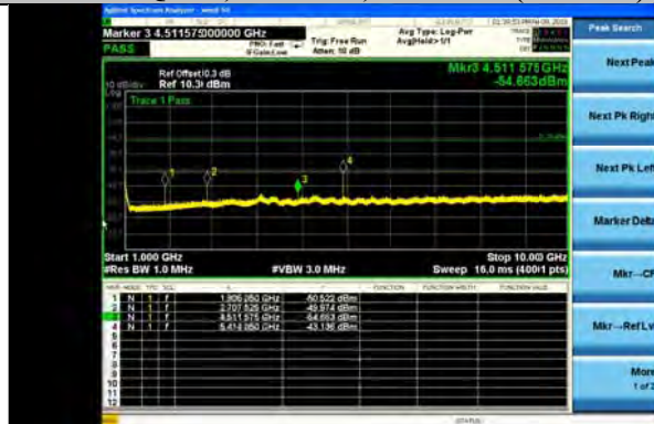
Mod: OQPSK, Mode 192, 915MHz (1-10GHz) Peak
