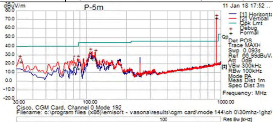
Title: TX Spurious Emissions from 30MHz-1GHz – Ch128 (927.8 MHz)
