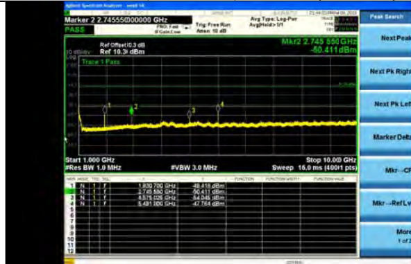
Mod: OQPSK, Mode 192, 927.8MHz (1-10GHz) Peak
