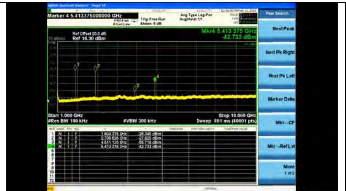
Modulation: 2FSK, Mode 96, 914.8MHz (1-10GHz)
