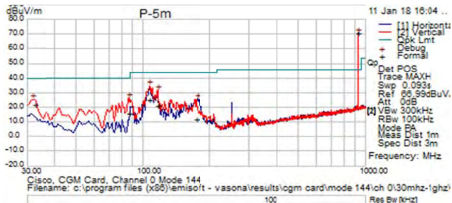
Title: TX Spurious Emissions from 30MHz-1GHz – Ch30(926.8 MHz)
