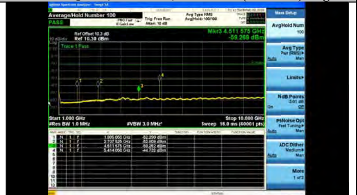
Mod: OQPSK, Mode 192, 915MHz (1-10GHz) Avg
