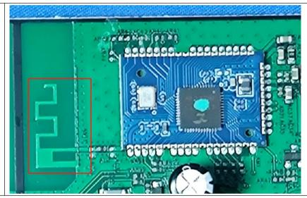
The antenna is PCB antenna.
