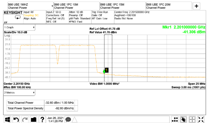
Figure 8.3-68: Conducted band edge emission at 2201 MHz, 5 MHz channel two-carrier operation (RBW = 1 MHz)
