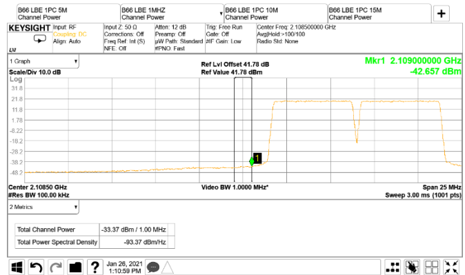
Figure 8.3-66: Conducted band edge emission at 2109 MHz, 5 MHz channel two-carrier operation (RBW = 1 MHz)
