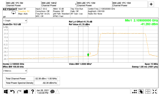
Figure 8.3-50: Conducted band edge emission at 2109 MHz, 5 MHz channel single-carrier operation (RBW = 1 MHz)
