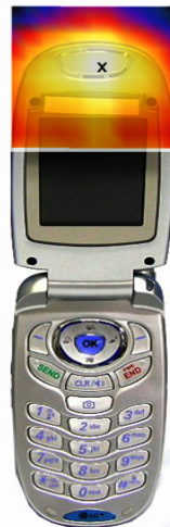
Figure 29 Sample E-field Scan Overlay
