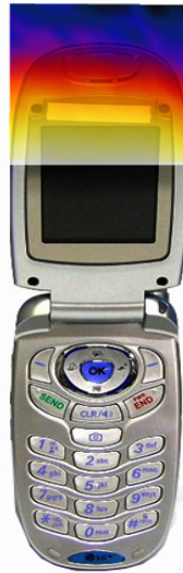
Figure 30 Sample H-field Scan Overlay
