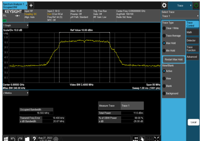
Plot 7-11. 26dB & 99% Bandwidth Plot Antenna WF5t (20MHz 802.11a (UNII Band 7) – Ch. 149, 12Mbps)
