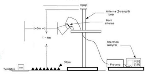
Above 18 GHz shall be extrapolated to the specified distance using an extrapolation factor of 20 dB/decade form 3m to 1m.
