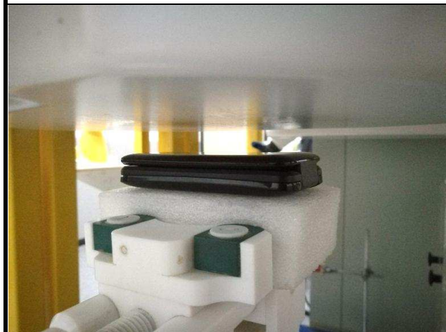
Front Face of EUT with 1.5 cm Gap
