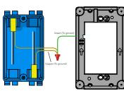
Install the mounting plate to the wall box and pull the rest of the wires through the mounting plate.
