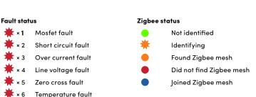
Flashing LED — Solid LED
