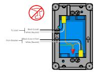
Identify and connect the wires to the back of the dimmer. Insert the wire into the terminal and secure it by hand-tightening the set screw.
