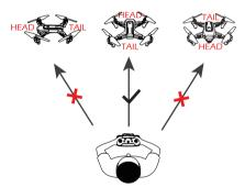
Please make sure the pilot to stay in the same orientation as the drone head faces when the drone is pairing.
