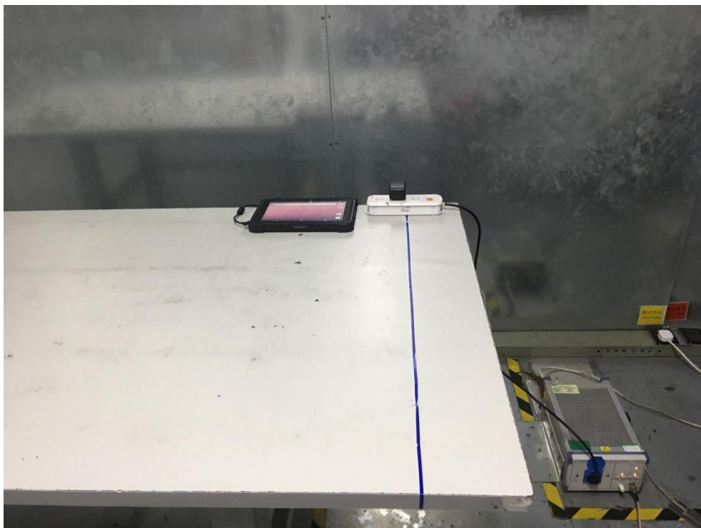
AC Conducted Measurement Photos
