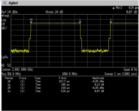
Duty Cycle = Ton / (Ton + Toff) =  $385[\mu s] / (385[\mu s] + 241[\mu s]) = 61.5[\%]$
