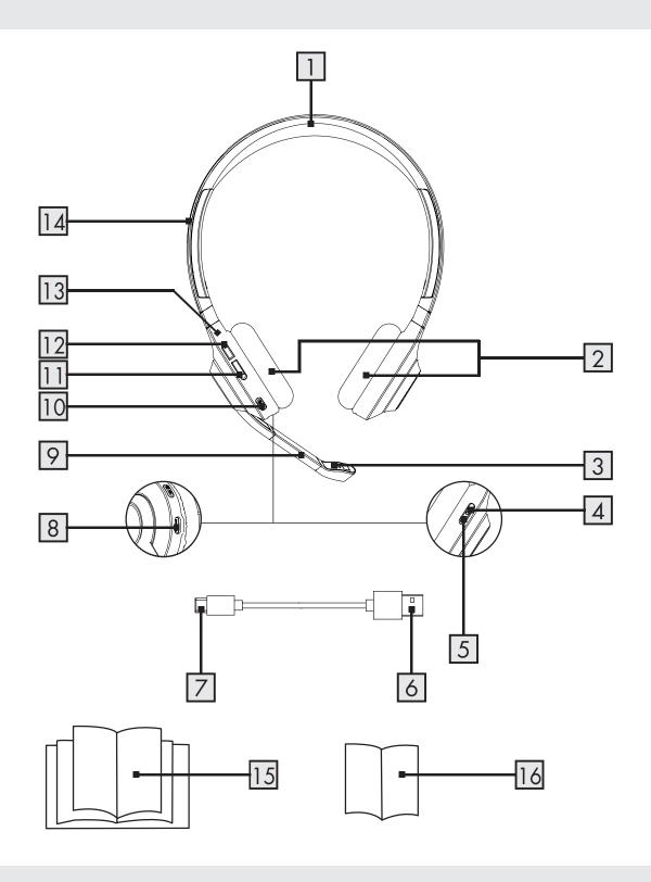
14 Magnetic attachment for microphone bracket on headband
