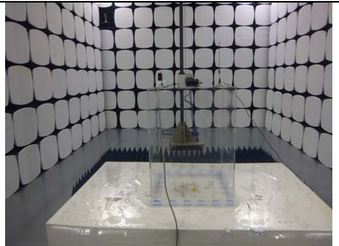
Radiated Spurious Emissions Test Setup Above 1GHz
