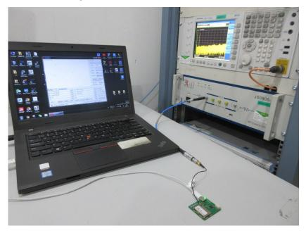
2 Radiated Spurious Emissions From 30MHz to 1GHz
