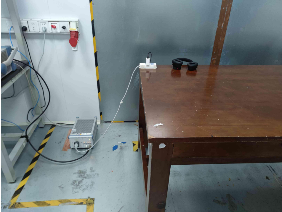
Conducted emissions at AC power line (150kHz-30MHz)
