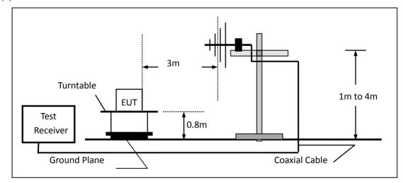
(c) For radiated emissions above 1000MHz
