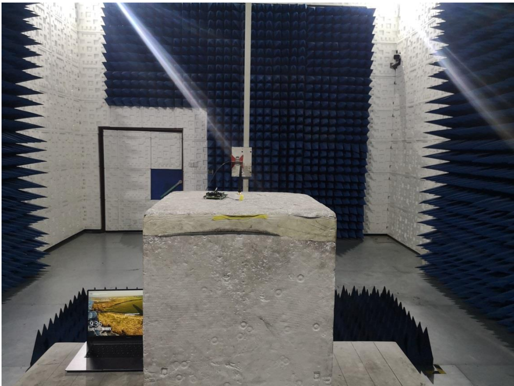
RADIATED EMISSION TEST SETUP ABOVE 1GHZ
