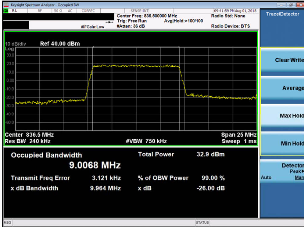
Plot 7-15. Occupied Bandwidth Plot (Band 26/5 - 10.0MHz QPSK - Full RB Configuration)
