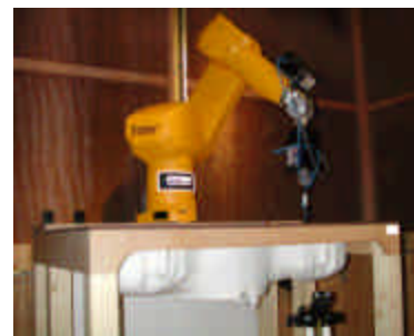
Figure 6.1 DASY4 Test System
