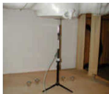
Figure 12.1 Dipole Validation Test Setup
