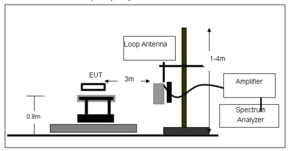
(B) Radiated Emission Test-Up Frequency 30MHz~1GHz
