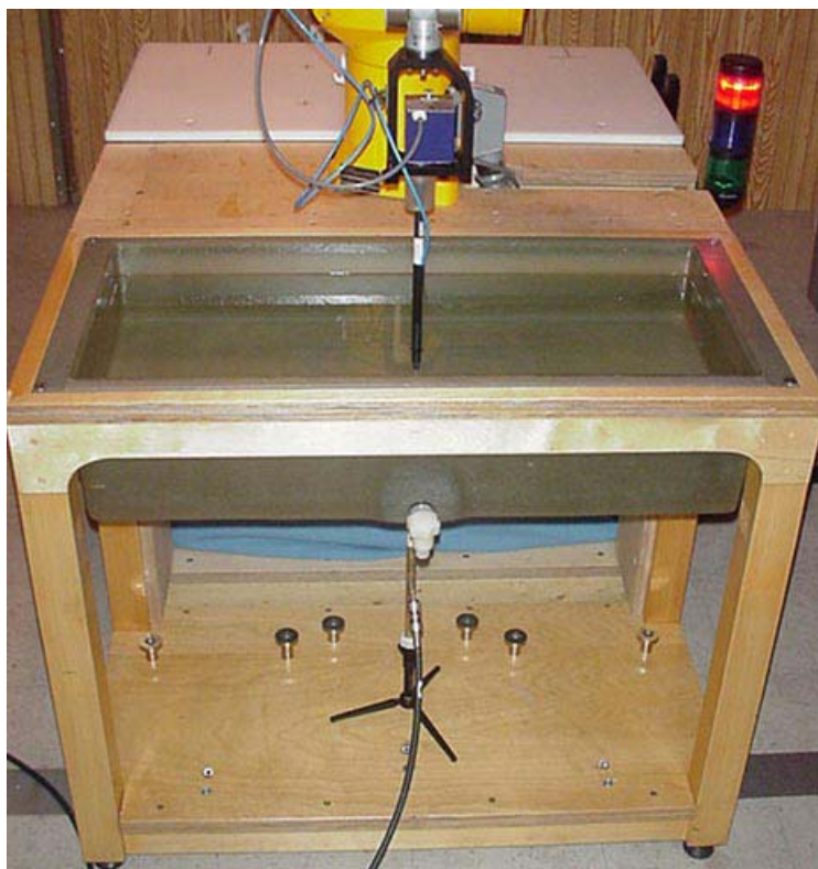
DASY4 SAR Measurement System with planar phantom
