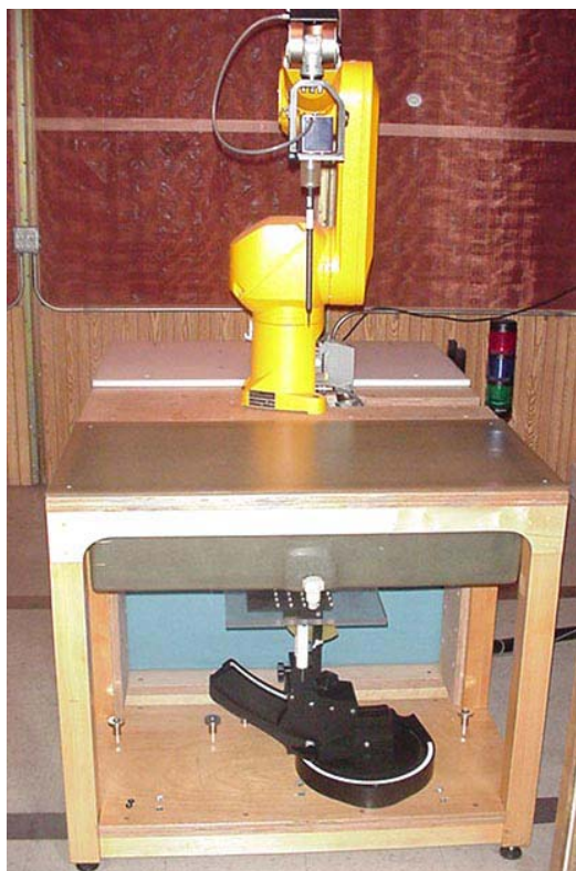
DASY4 SAR Measurement System with planar phantom
