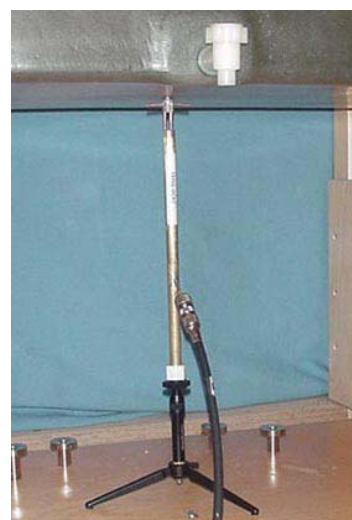
2450MHz Dipole Setup
