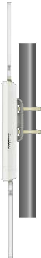
1. Position the C260-X unit in the desired location on the pole.
