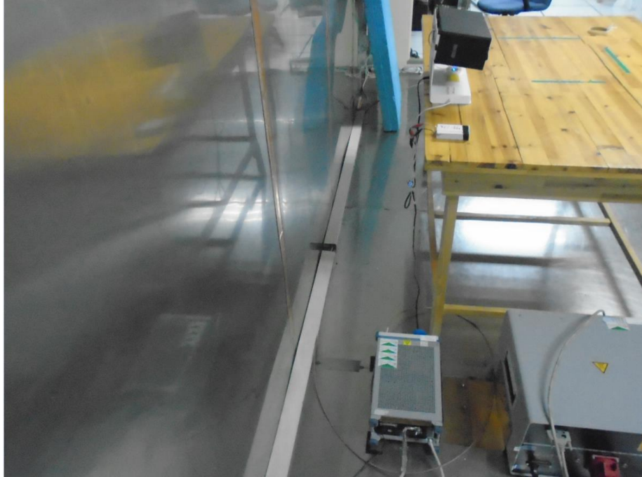
Photograph 1: Set-up for measurement of conducted emission
