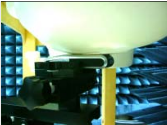
Figure 14. Right Head SAR Test Setup (Cheek)
