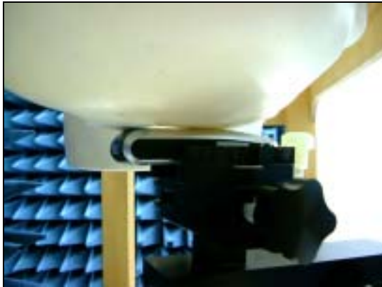
Figure 12. Left Head SAR Test Setup (Cheek)
