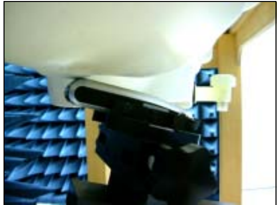
Figure 13. Left Head SAR Test Setup (Tilted)
